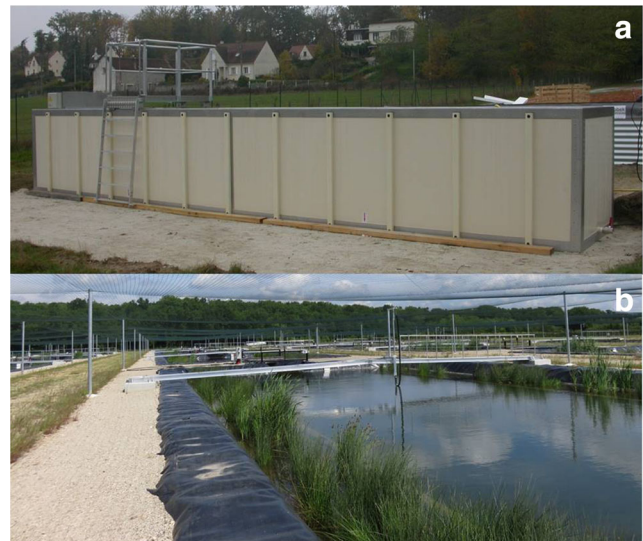
Fig. 6 Examples of PLANAQUA experimental facilities. a Mesocosms equipped with beaters to generate waves ( left part of the mesocosm ) and transparent covers to generate a greenhouse effect to increase surface water temperature (not shown). Each mesocosm is 10 m long, 1.7 m large, and 1.5 m deep. The angle and frequency of the wave beater can be automatically manipulated within a range allowing for subsurface wave and water stratification to full water mixing. The percentage of surface cover can vary manually from 0 to 100 %. This system makes it possible to investigate effects of water turbulence on the fate and effects of contaminants. b Artificial lakes equipped with buoys installed on footbridges. Each lake constitutes a miniature replicate of a natural shallow pond integrating littoral, benthic, and pelagic zones, the spatial structure of the landscape can be manipulated to some extent, and real-time biophysical data are automatically recorded down to the temporal scale of a few minutes. To our knowledge, such highly replicated and instrumented systems have no analogue elsewhere in the world
