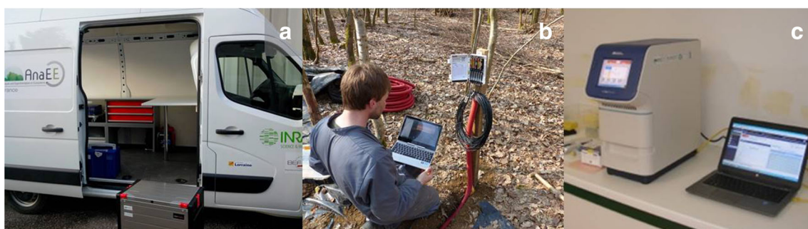
Fig. 8 The Mobile Platform for Observation and Experimentation in Terrestrial Ecosystems (E). a View of the truck. b Monitoring of soil water content using decagon probes. c qPCR device
